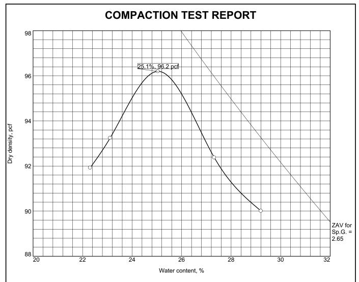
Test specification: ASTM D 698-12 Method A Standard
